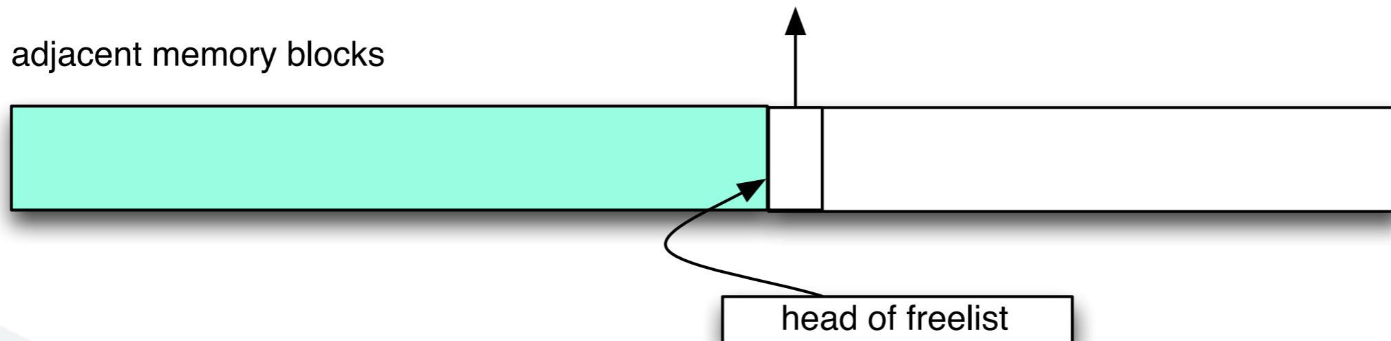
allocated block overflowing into free one
